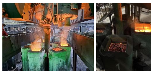
Fig. 6 Different powder behavior in molds from the same casting plate
