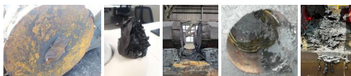
Fig. 4. (a) Massive, vitrified slag residue detected in the hot top area; (b) positioning of the ingots inside the reheating furnace; (c-d) vitrified residue mixed with scale present on specific furnace components
