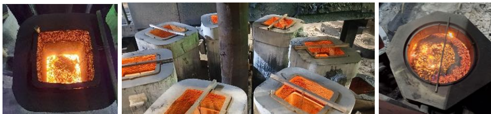
Fig. 5 No completed filling and already exposure of the bath surface
