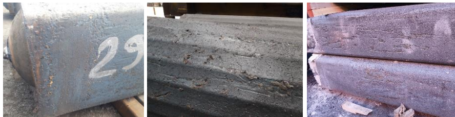
Fig.1 Surface irregularities detected during visual inspection of as cast ingots
