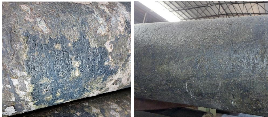
Fig.3 – Surface of superalloys ingots cast with powder E (left) compared to powder F (right).
