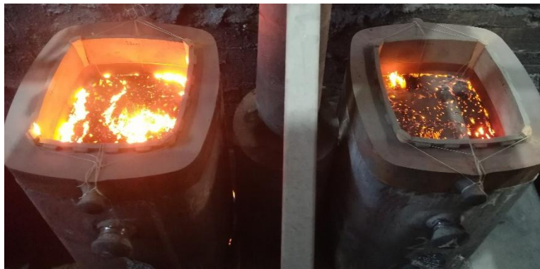
Fig.1 – Powder A behavior (left) compared to powder B (right) during casting.
