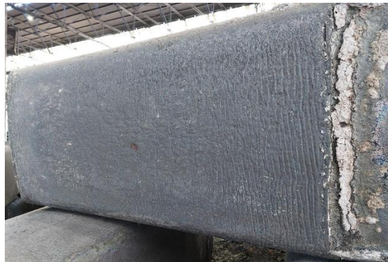
Fig.2 – Austenitic ingot cast with powder C.
