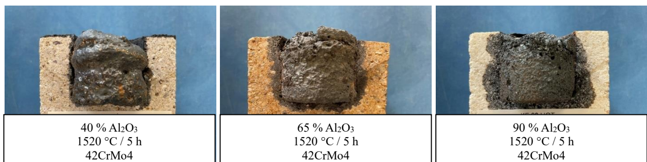
Fig. 1 – Cup Tests (Steel) with various refractory grade
