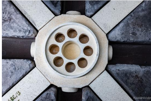
Fig. 2 – Inside view of the innovative SmartCast-Spiderbrick
