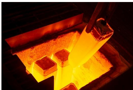
Fig. 8. Photograph from current full-scale operation at Ovako reheating with 100% hydrogen as a fuel.
