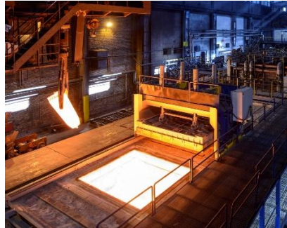
Fig. 2. Discharge of a heated stainless steel ingot from a soaking pit furnace fired with flameless oxyfuel at Alleima in Sweden.
