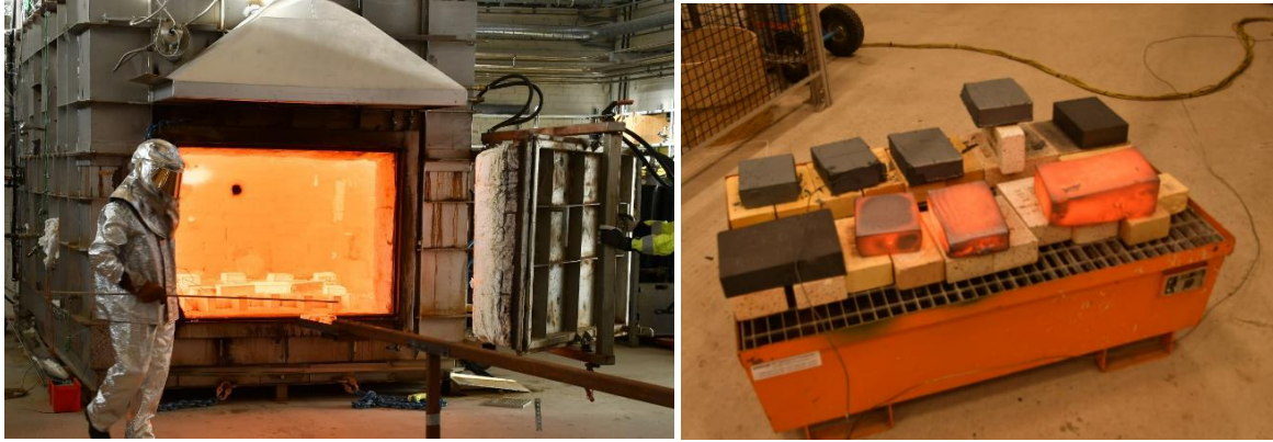
Fig. 6. Laboratory tests with 100% hydrogen as a fuel using 10 kg samples of various steel grades at Linde's Technology Center in Stockholm, Sweden.
