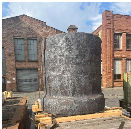
Fig. 5 -Single piece forged skull crucible ready for machining.
