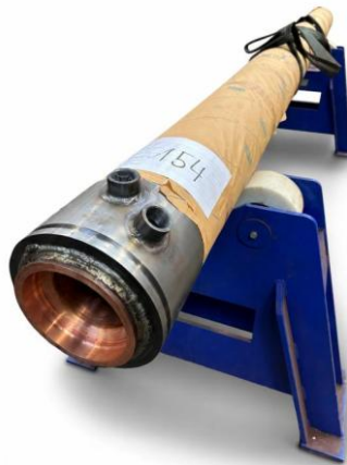
Fig. 4 - Example of a copper power ram for VAR/ESR applications
