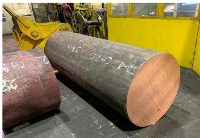
Fig. 1 - Large copper-alloy billet used as starting material for forged remelting components; billet diameter is approximately 900–1,000 mm and piece weight can reach 17 t
