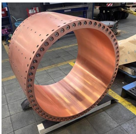
Fig. 7 - Short collar mould concept for ESR applications; deep-drilled and slotted cooling configurations.
