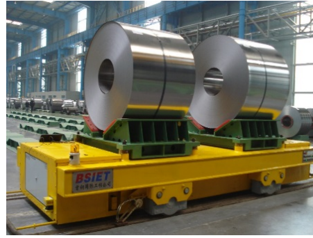
Fig.5 Steel coil transport car with non-contact power supply
