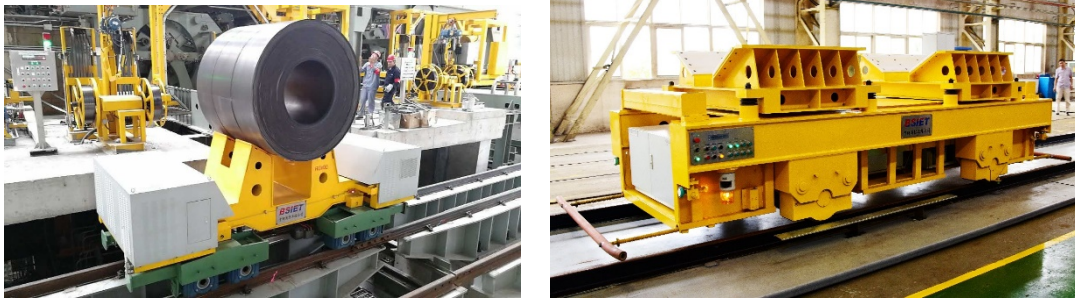
Fig.8 Steel coil transport car with supercapacitor power supply
