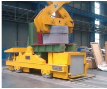
Fig.5 Steel coil transport car with non-contact power supply
