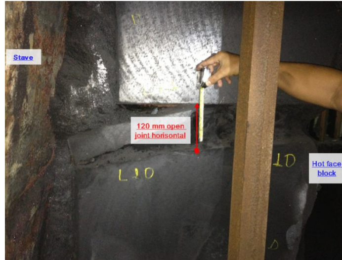
Fig. 1: Expansion due to alkali penetration.
