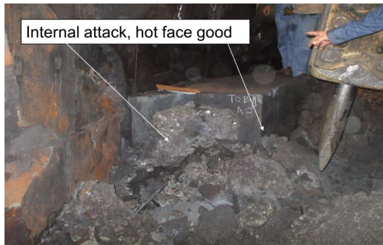
Fig. 3: Example of iron and slag penetration into a carbon refractory lining.
